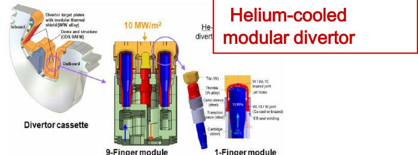
Thimbles tested at  $12 \text{ MW.m}^{-2} \leq 200$  cycles
