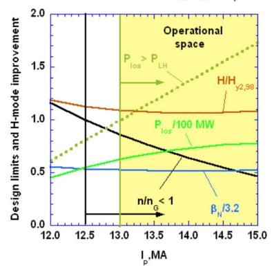
Hybrid mode of operation: I>13MA, Pfusion 250 MW, H~1,1 but only pulse length only 1000s
