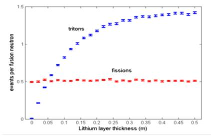
Fissions and bred tritons per fusion-born neutron as a function of lithium layer thickness. Here the uranium layer is 15 cm thick, and the 6Li enrichment is 90%. Kf~constant
