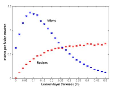
UO2 pebble layer thickness 18 cm Li-Pb layer thickness 25 cm Li enrichment 90% Li atomic fraction in Li-Pb 10% Fission ratio Kf 0.47 M ~7.7 Tritium breeding ratio 1.05
