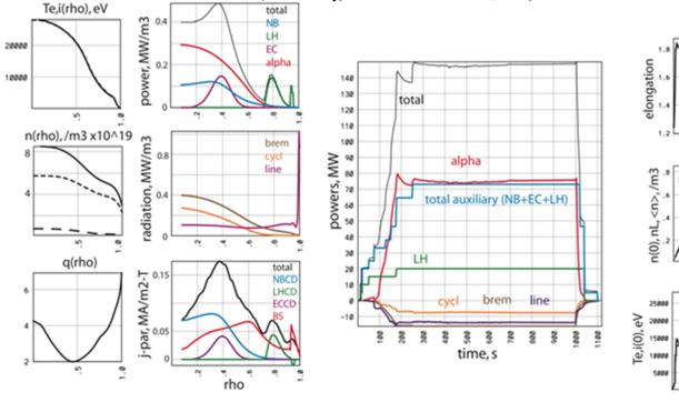
The steady state scenario consumes about 85-100 Wb to ramp up the plasma current to 7.5-10 MA, with external heating and current drive assisting.
