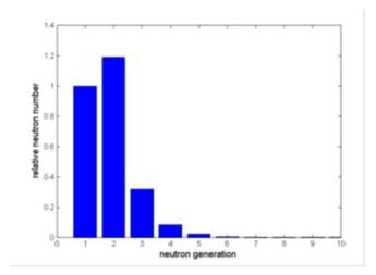
In a deeply subcritical blanket the fate of fusion 14 MeV neutrons determine the characteristics of the blanket. Total number of secondary neutrons ~1.7 per a fusion neutron is small.
