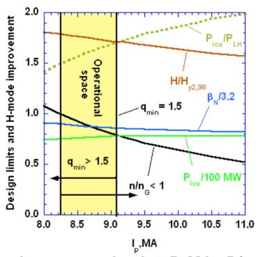
Steady state mode : I~8,5 MA , Pfusion=` 250 MW , Q=5 ,  $\beta$ N<1.5 but H = 1,7. In the range of 8-10 MA, to get a Q of 3-6 and fully not inductive current drive the
