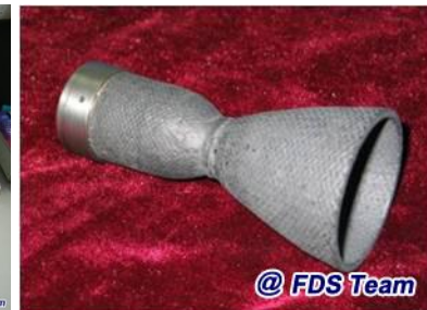
Connection of metal and SiC composite
