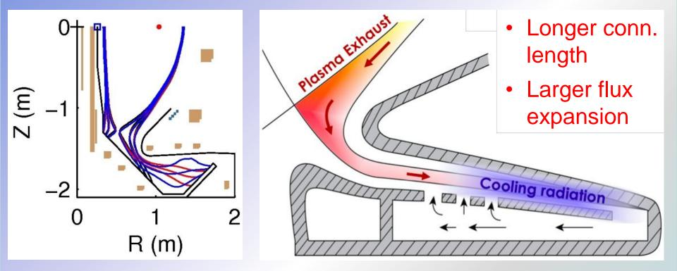
Critical issue: DEMO compatible coils to establish configuration
